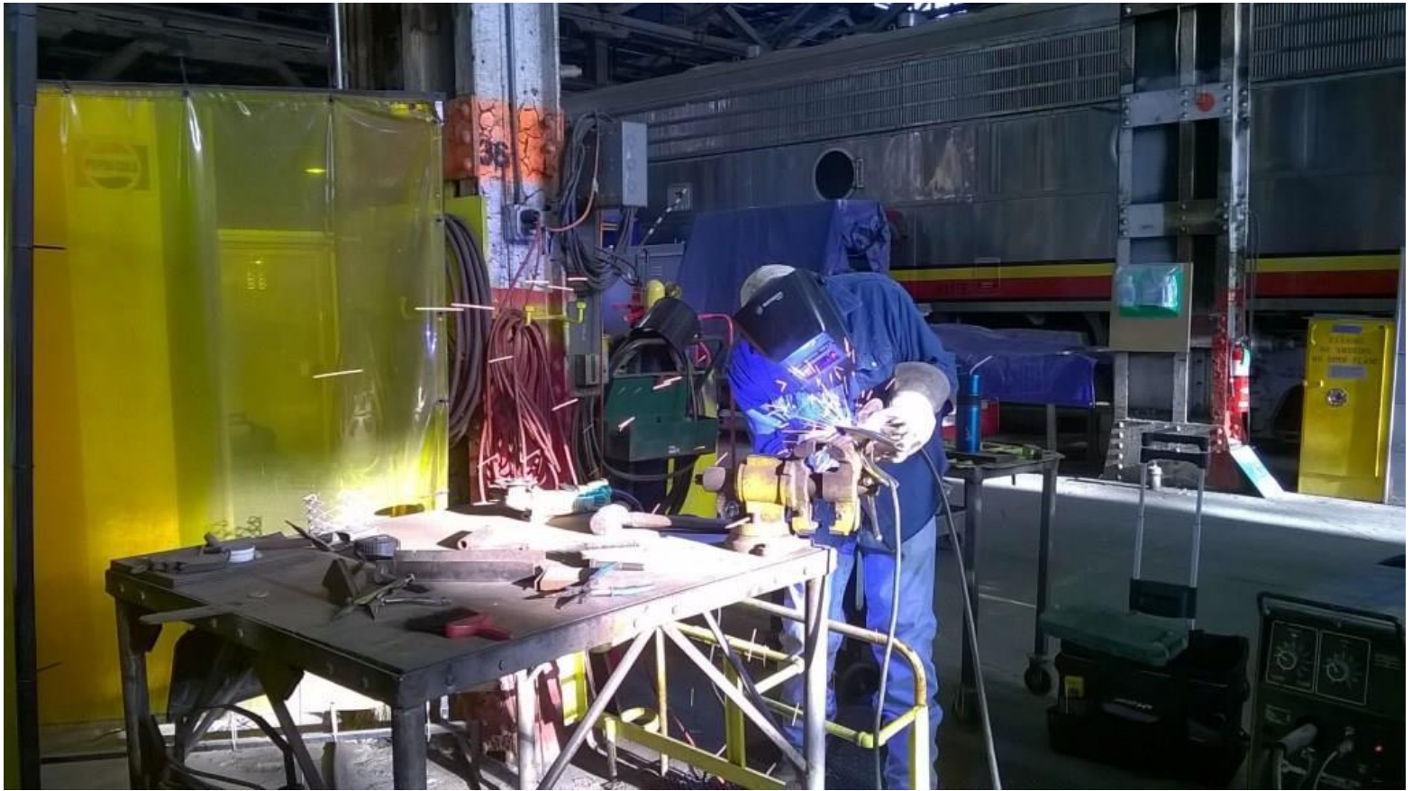
Cliff makes new securing clamps for the chipper and his cart
